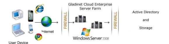
There are three different types of machines (or Virtual Machine). In the smallest deployment unit, the three different logical nodes can co-exists in one single machine.
